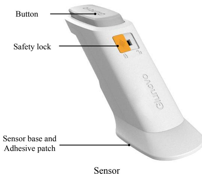
The continuous glucose monitoring sensor is a product with a sterile sealed pouch. The sensor is mainly made up of an applicator, a sensor base and a sensor electrode. The base consists of a PC base and an adhesive patch. Insert the sensor electrode into the subcutaneous tissue of the abdomen and remove the applicator. The base is attached to the abdomen for up to 14 days of monitoring. Please discard disposable sensor after wearing.
